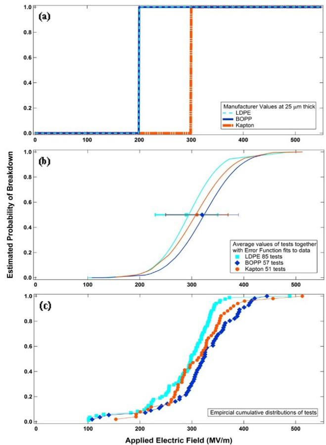
**Fig. 1.** Successively more accurate representations of dielectric strength for LDPE, BOPP, and PI (Kapton). (a) Manufacturer values [17-19]. (b) Averages and standard deviations with underlying error function fits to USU step-up tests. (c) Empirical cumulative distributions of USU step-up tests.
