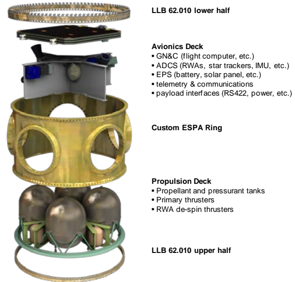
Figure 5: The Andrews SHERPA platform is a modular spacecraft bus that leverages the Avionics Deck and Propulsion Deck currently being developed for the SHERPA in-space tug.
