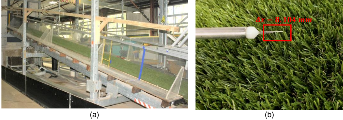
Figure 2 – (a) Experimental chute with dense coverage of grass; (b) WRL dual-tip conductivity probe
