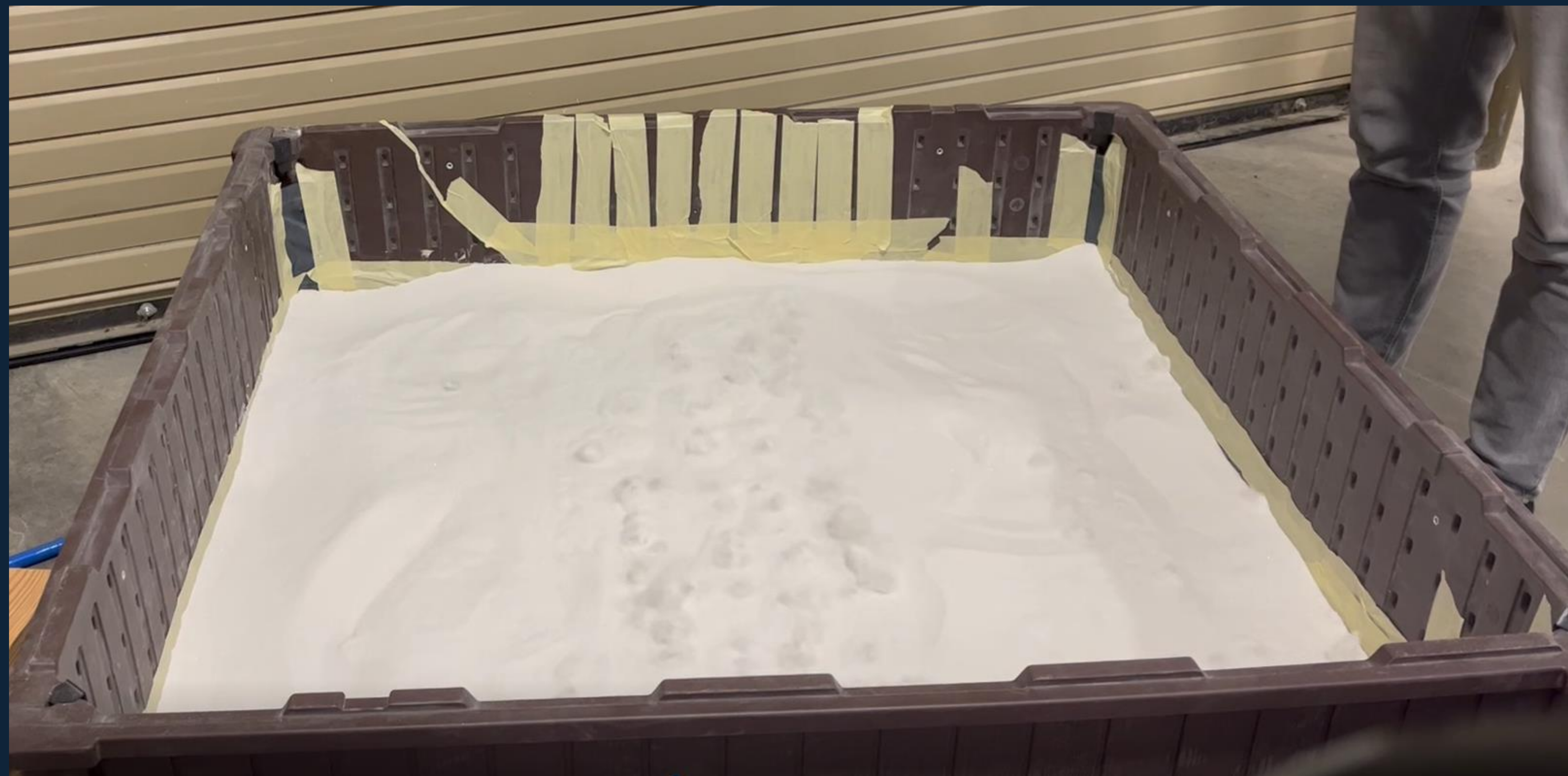
Liquid sandbox used for testing the thermal properties of wireless charging systems. Bubbling is visible in the middle of the sandbox where the sand is acting as a liquid.
