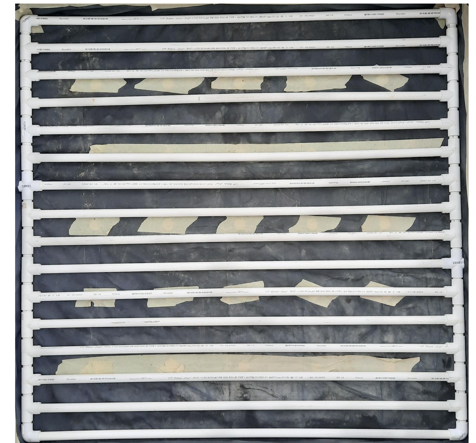
PVC pipe grid has 2000 small holes that allow air to leak out and flow upward through the sandbox creating liquidization
