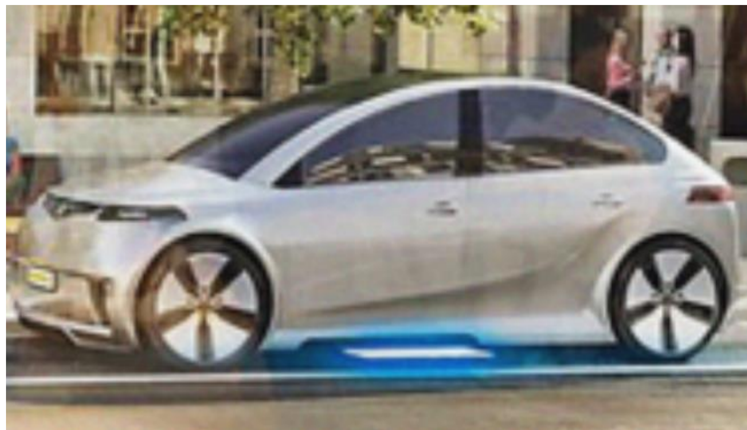
Simulated image of car being charged as it drives. Blue glow added for emphasis to show transmitter coil
