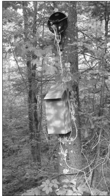
Figure 2. A howl box unit consisting of an outdoor speaker and parabolic microphone for recording.
