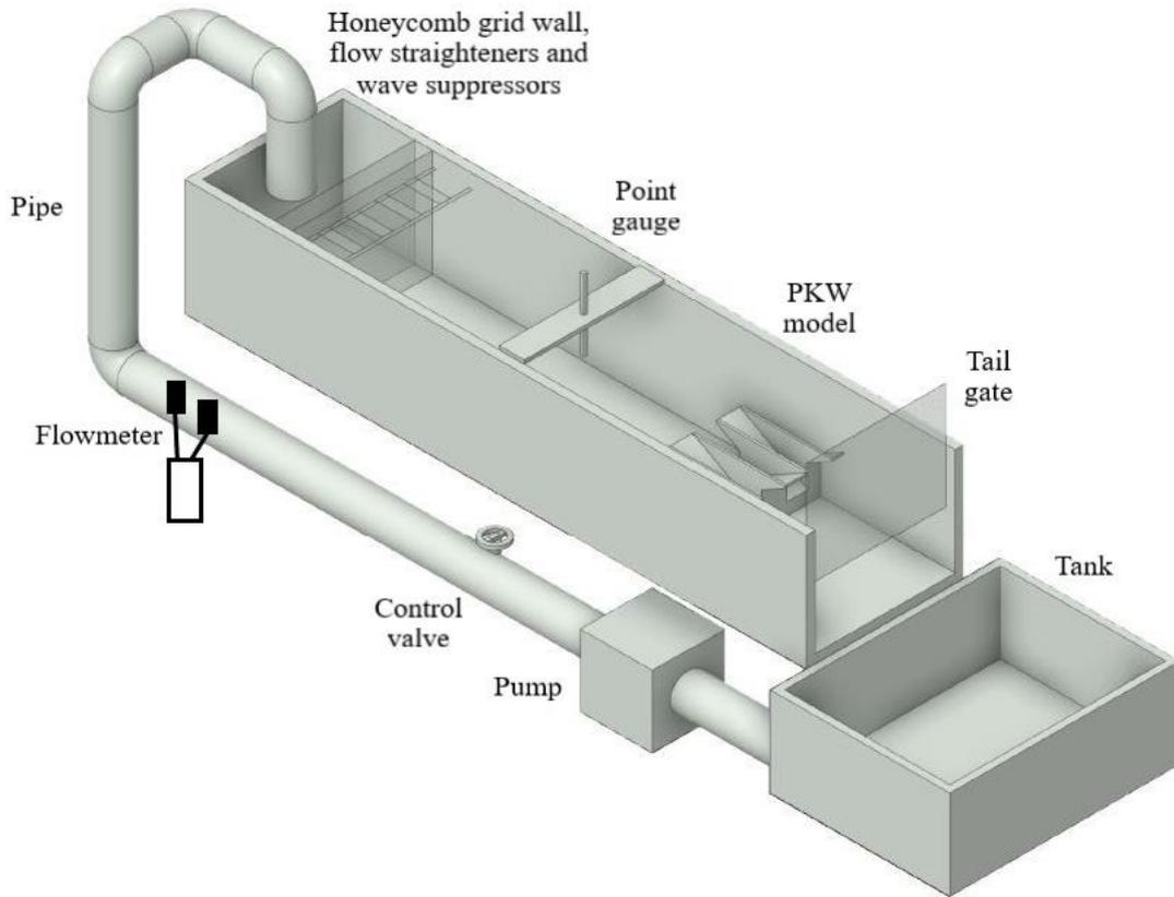
Figure 3 - Schematic of the experimental setup.
