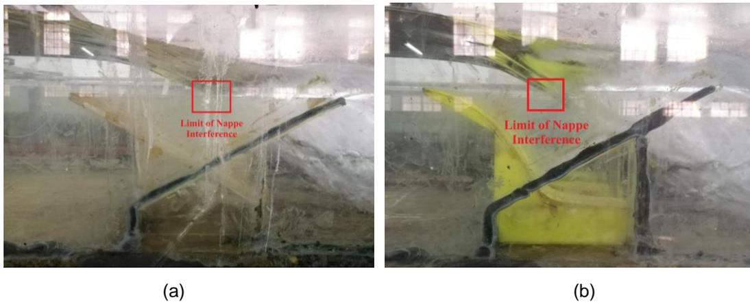
Figure 6 - Limit of nappe interference for  $Q_{PKW} \approx 3 \times 10^{-2} \text{ m}^3/\text{s}$  (a) PKW-L at  $H/P = 0.76$ ; (b) PKW-CL at  $H/P = 0.73$ .
