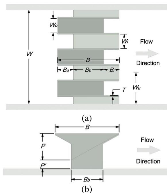
Figure 1 - Typical geometry of PKW: (a) plan; (b) side-elevation.
