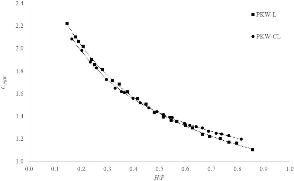
Figure 4 -  $C_{PKW}$  versus  $H/P$  data for PKW-L and PKW-CL weirs.
