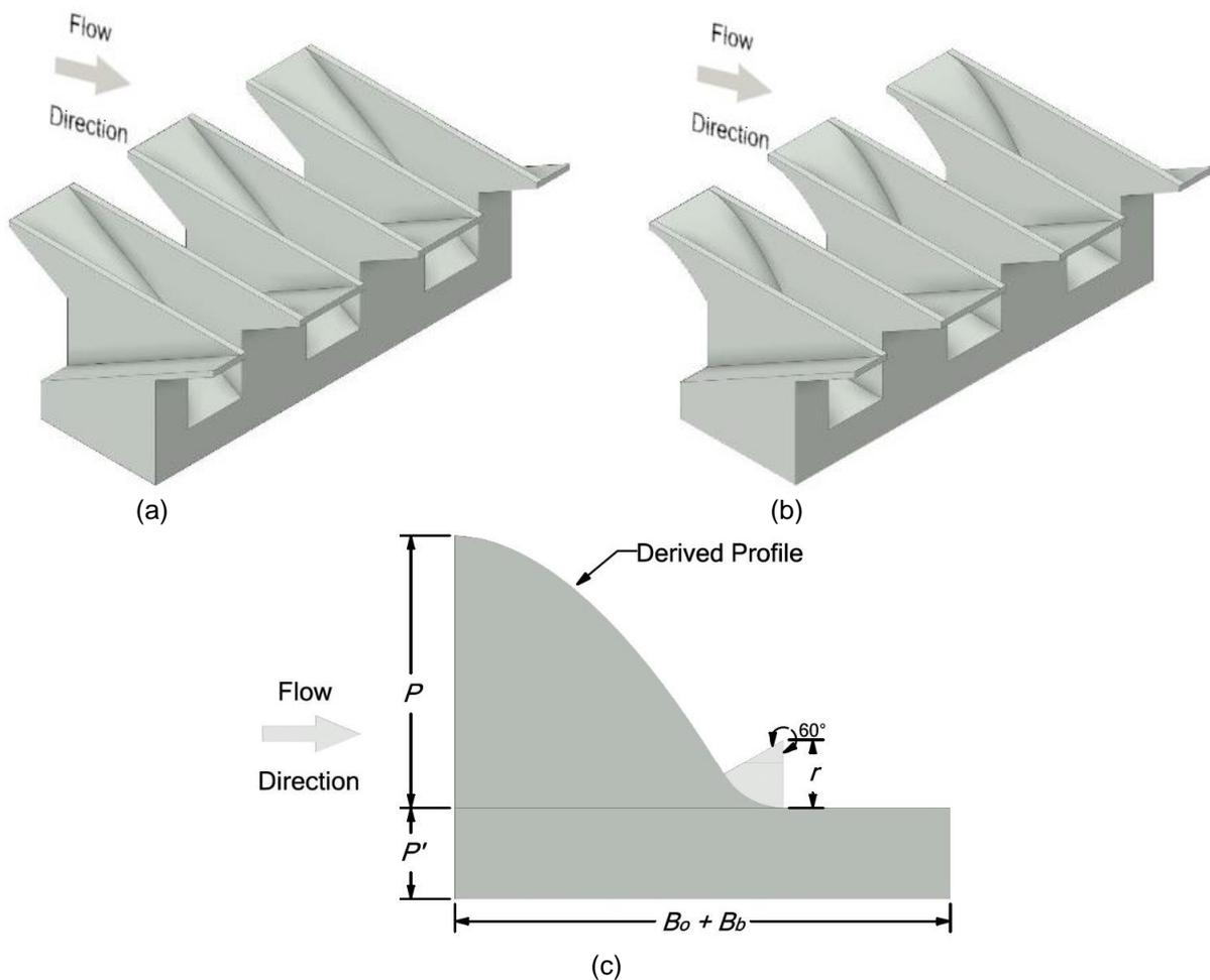
Figure 2 - (a) Overview of PKW-L weir model; (b) overview of PKW-CL weir model; (c) profile of outlet key for PKW-CL weir model.
