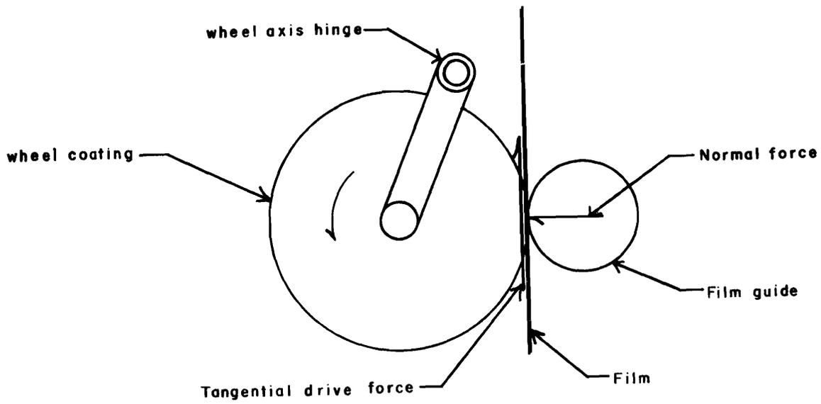
Figure 4. Diagram showing operation of and forces acting on the coating wheel before any modifications.
