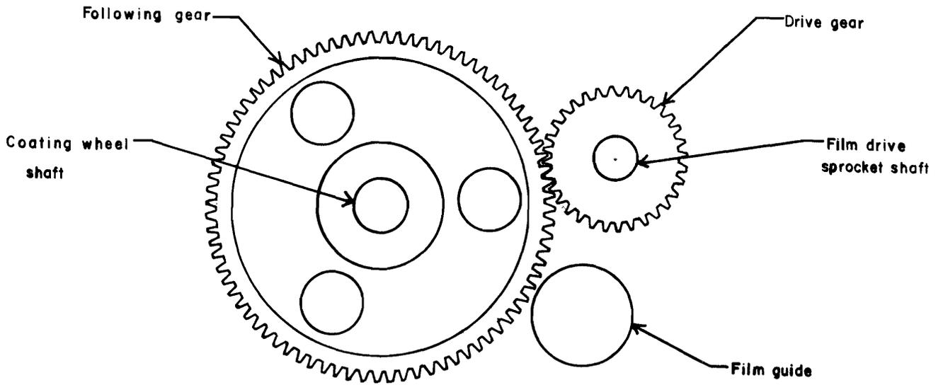
Figure 6. Spur gear configuration.
