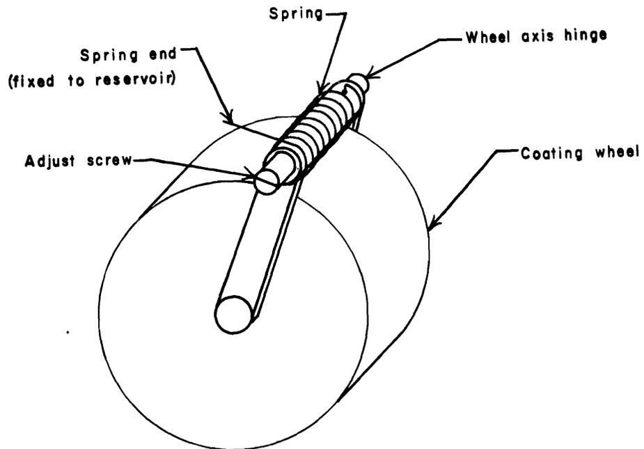
Figure 5. Sketch of the coating wheel assembly modified by the addition of a helical spring to increase the normal force.
