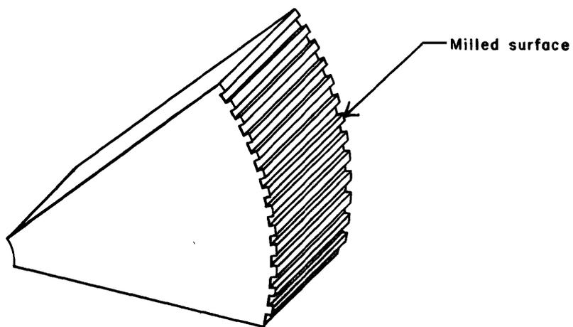
Figure 3. An enlarged section of the coating wheel.
