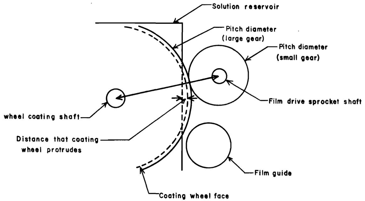
Figure 7. Sketch showing the location of the coating wheel shaft.
