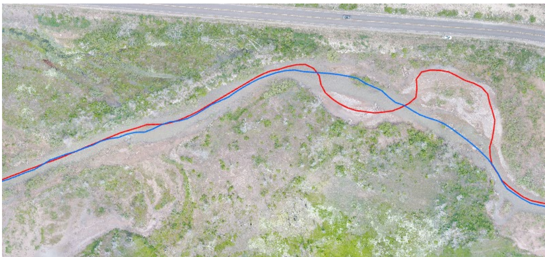
Figure 11. Two Meander Cutoffs, Pre-flood (red) and post-flood (blue) centerlines
