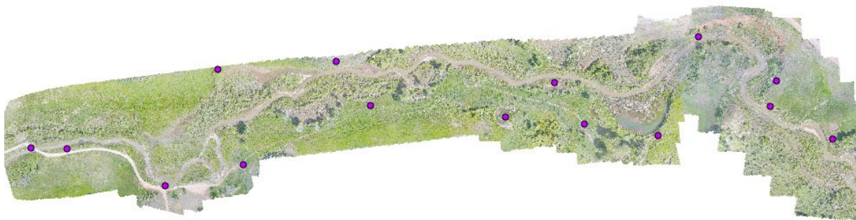
Figure 3: Control Points (pink) Overlaying the 06/09 Drone Imagery on the Lower Diamond Fork River.
