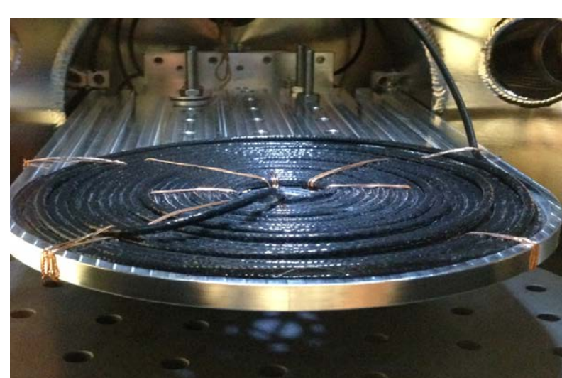
Fig. 5. Cabling Under Testing in SST
