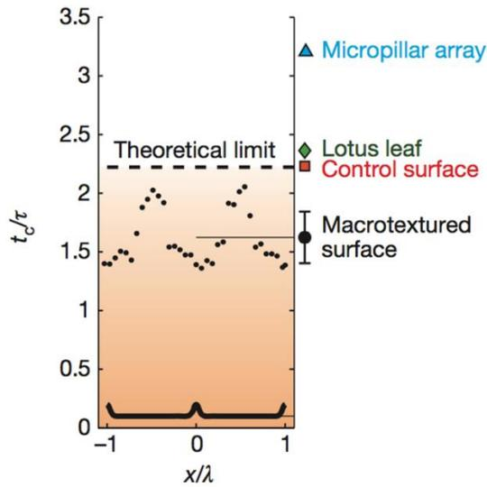
**Figure 5:** From Bird et al 2013 [1.] The y-axis shows non-dimensional time as obtained from Equation 1. The x-axis is non-dimensional distance, representing how far from a ridge the droplet impacted the surface. On the right is shown contact times of other comparable surfaces. Lotus leaves are naturally superhydrophobic and seen as a standard to beat.
