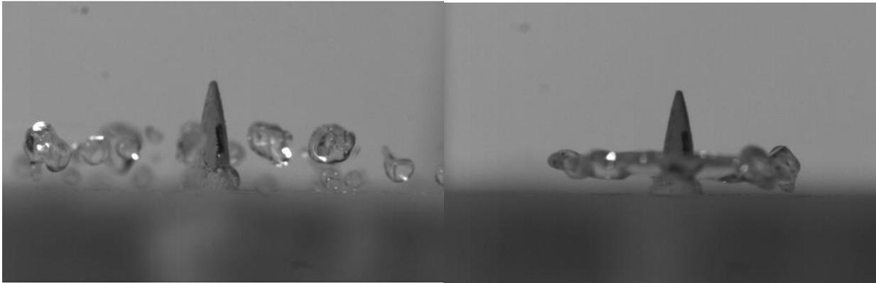
**Figure 4:** The frame on the left is of a droplet rebounding after falling from a height of 32 inches. The droplet has split into countless smaller droplets, some of which never fully leave the surface. On the right, the droplet fell from only 8 inches and there is a clear frame of liftoff since the droplet rebounded without splitting apart.
