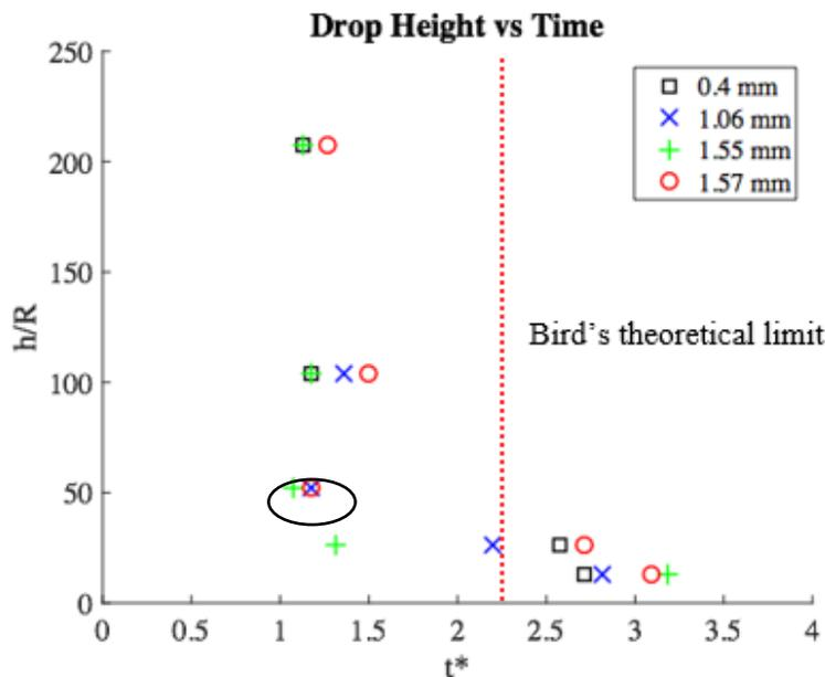
**Figure 6:** The y-axis shows drop height,  $h$ , non-dimensionalized using droplet diameter,  $R$ . The x-axis is non-dimensionalized time gotten from Equation 1. The different shapes depict different needle sizes. The largest needle, represented by red circles was triangular. It should be noted that each cluster of data points represents a drop height. Heights of 2, 4, 8, 16, and 32 inches were tested. The needles in this study achieved 50% contact time reduction at best.
