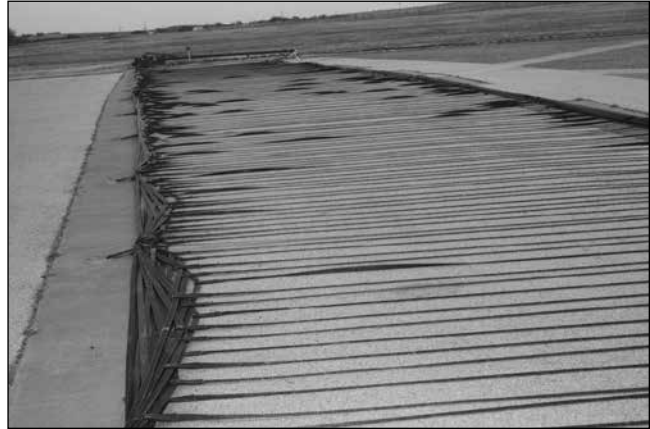
Figure 1. BAK-15 Barrier Arresting System as it lies ready for deployment on a military airstrip.
