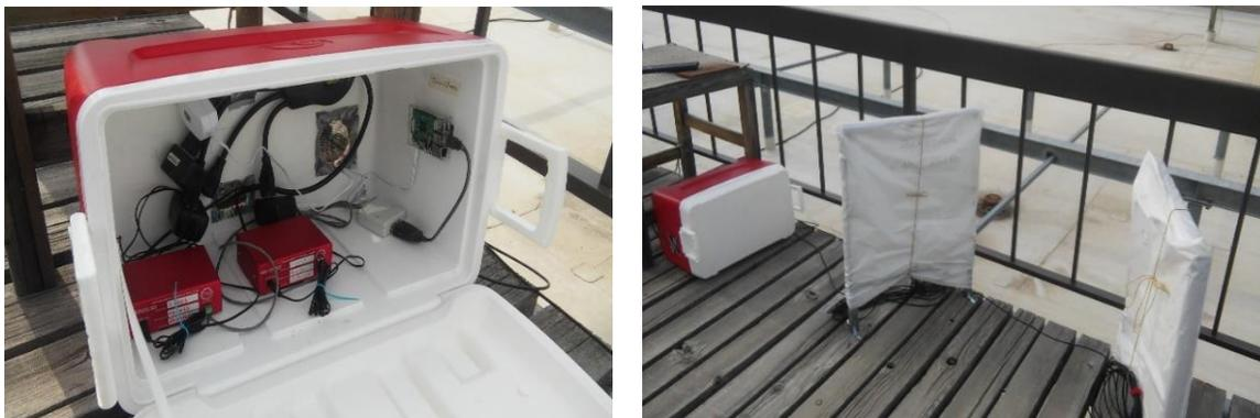
*Figure 2. Experimental equipment placed inside the cooler for weather protection (left). Set up of the equipment at the rooftop of the Science and Engineering Research Building (right)*
