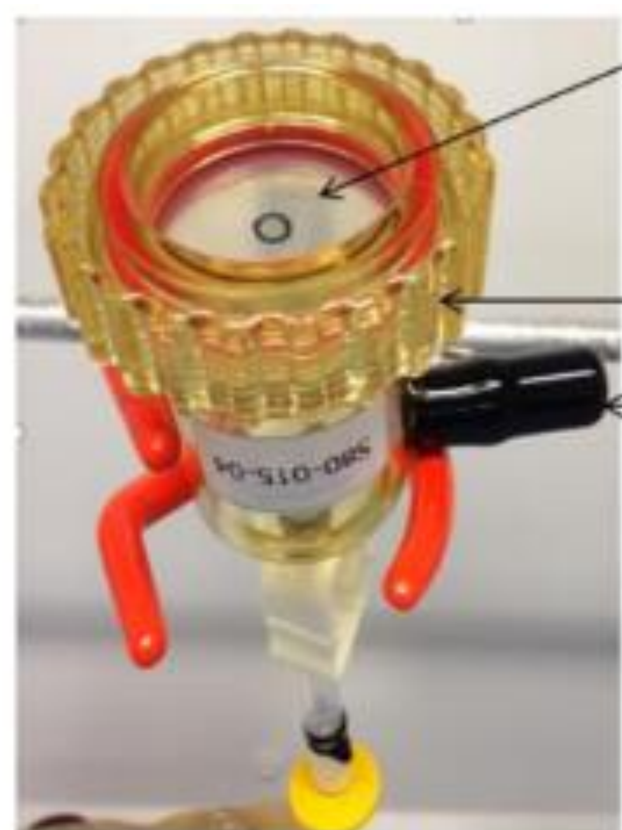
Figure 1. Test unit used in aerosol microbial ingress test [1]. The unit was filled aseptically with TSB using the black line.
