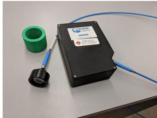
**Figure 3: Ocean Optics HR4000 spectrometer with fiber optic cable and collimating lens**
