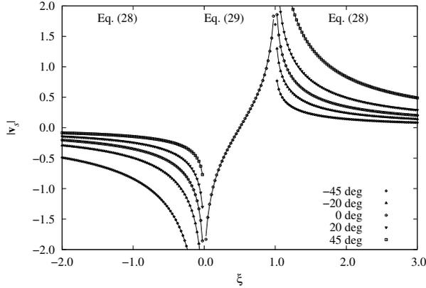
**Figure 5. Magnitude of induced velocity along points collinear with the bound portion of the vortex sheet.**
