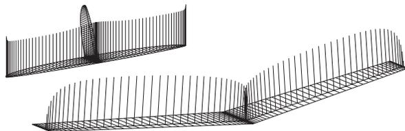
**Figure 13. Circulation distribution for a system of interacting lifting surfaces.**
