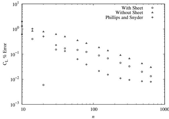
**Figure 9. Percent error of the lift coefficient as a function of grid resolution.**
