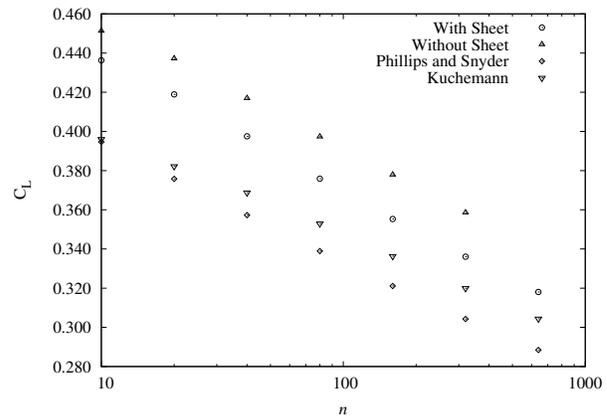
**Figure 11. Lift coefficient for a wing of aspect ratio of 8 with 45 degrees of sweep as a function of grid resolution.**
