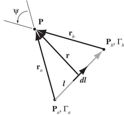
Figure 2. Position vectors showing the geometry for a vortex line segment with varying strength.
