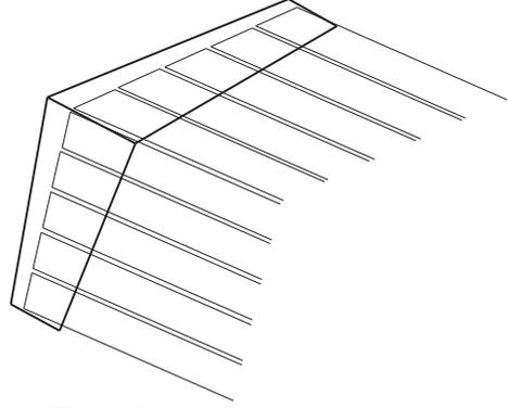
**Figure 6. Horseshoe vortex sheet distribution along quarter chord of lifting surfaces.**
