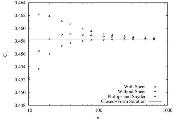
Figure 8. Lift Coefficient as a function of number of discretization elements for an elliptic wing with aspect ratio  $32/\pi$ .
