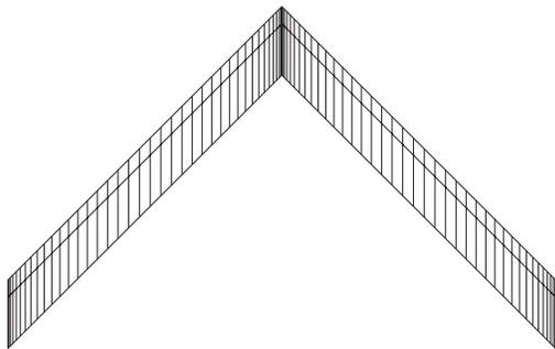
**Figure 10. Rectangular wing with aspect ratio of 8 and 45 degrees of sweep.**
