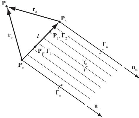
Figure 1. Position vectors and geometry for a horseshoe vortex sheet.
