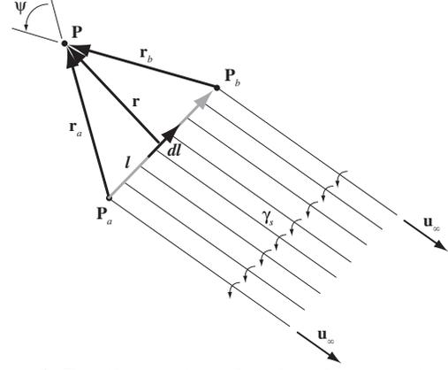
**Figure 3. Position vectors showing the geometry for a semi-infinite vortex sheet with constant strength.**
