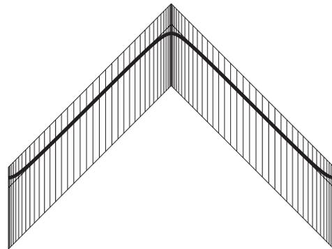
**Figure 12. Lifting-line distribution based on the work of Kuchemann showing first-order continuity at wing plane of symmetry.**
