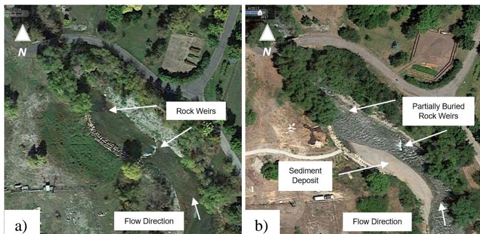
Figure 5 – Blacksmith Fork River Rock Weirs in (a) 2014 and (b) 2017 (Google, n.d.).
