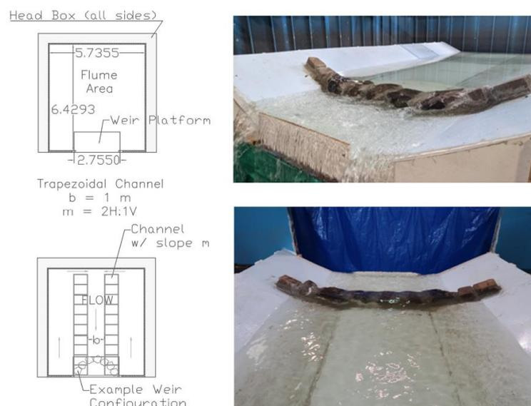
Figure 3 – Flume plans (lengths in m) and laboratory setup with flows of 30 L/s (top right) and 50 L/s (bottom right), photos courtesy K. Margetts.
