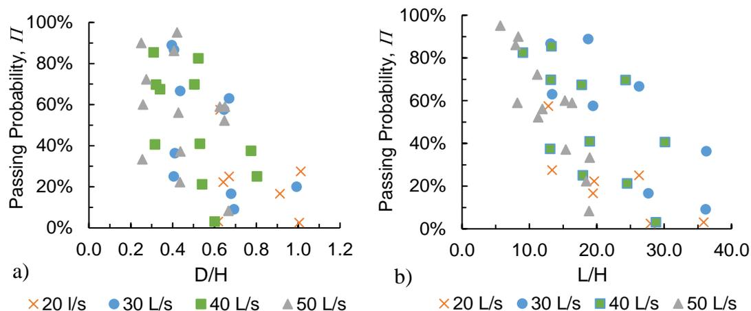
Figure 4 – Passing Probability versus (a)  $D/H$  and (b)  $L/H$  at  $Q= 20$  L/s, 30 L/s, 40 L/s, and 50 L/s.
