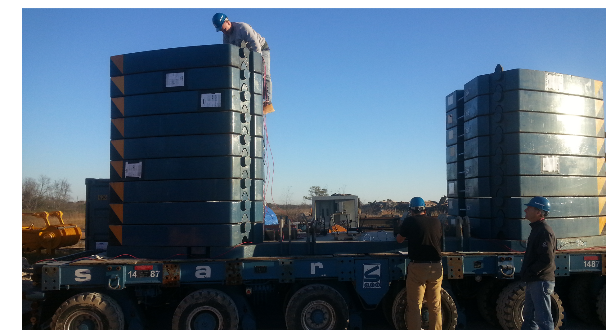
Placing the accelerometers on the loaded SPMT.
