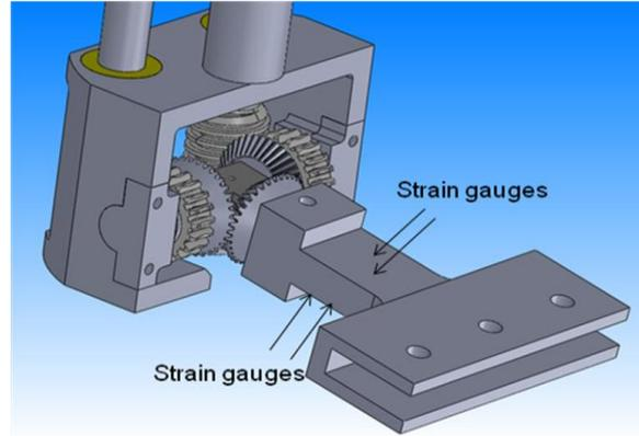
**Figure 5. Strain gages are mounted at the wing root.**
