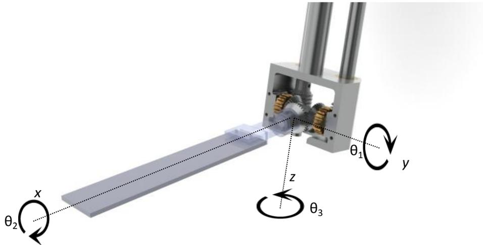
**Figure 1. Coordinate definitions of the flapping wing mechanism.**
