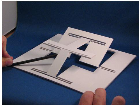
Figure 3: A Planar Four-bar Lamina Emergent Mechanism made from Polypropylene
