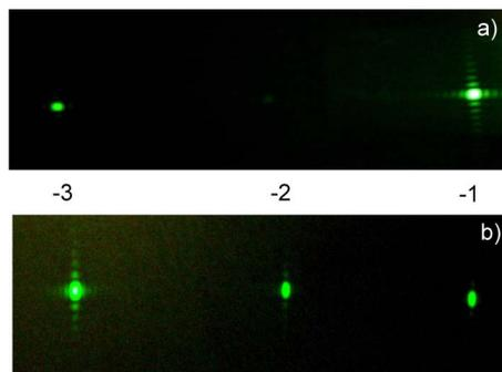
Fig. 6. Photographed images of the diffracted orders corresponding to the spectra shown in Fig. 5. (a) For the structure considered in Fig. 5(a), the cancellation of the  $-2$  order is evident; (b) for the structure considered in Fig. 5(b), a clear intensification of the  $-3$  order is observed.
