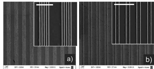
Fig. 3. Detail of the fabricated dual-period nanostructures. Ni wires 25 nm thick and total length  $\approx 5 \mu\text{m}$  were deposited on a  $\text{SiO}_2$  film. (a)  $J = 5$ ,  $M = 25$ ,  $d = 270$  nm, and  $D = 2625$  nm. Scale bar in the inset is  $2 \mu\text{m}$ . (b)  $J = 2$ ,  $M = 39$ ,  $d = 890$  nm, and  $D = 2670$  nm. Scale bar in the inset is  $4.5 \mu\text{m}$ .
