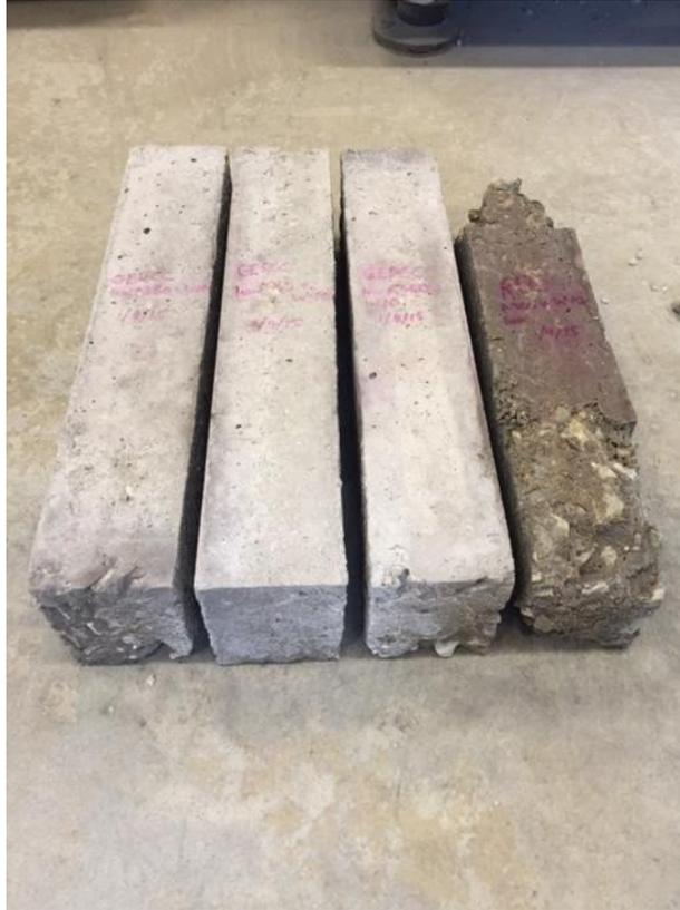
Figure 6. Freeze Thaw Samples After 300 Cycles
