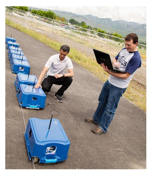
"We use the robots to look at the security of control algorithms," said Gerdes. "What actually determines how a vehicle reacts to what's happening in front of or behind it? The control algorithm tells the vehicle what the car in front of it is doing. If the lead car accelerates, it tells your car to accelerate at a specific speed."
