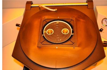
Fig.2 Chuck and mask holder for the backside alignment system
