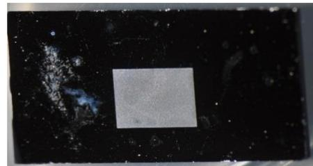
Fig.3 An etched hole on the backside of the Si wafer.
