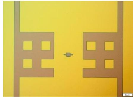
Fig.5 The absorber (center) was coated with  $Al_2O_3$  and Fe.
