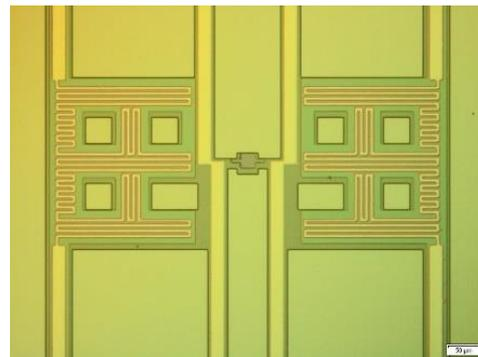
Fig.7 Patterns defined by photolithography in step-10.
