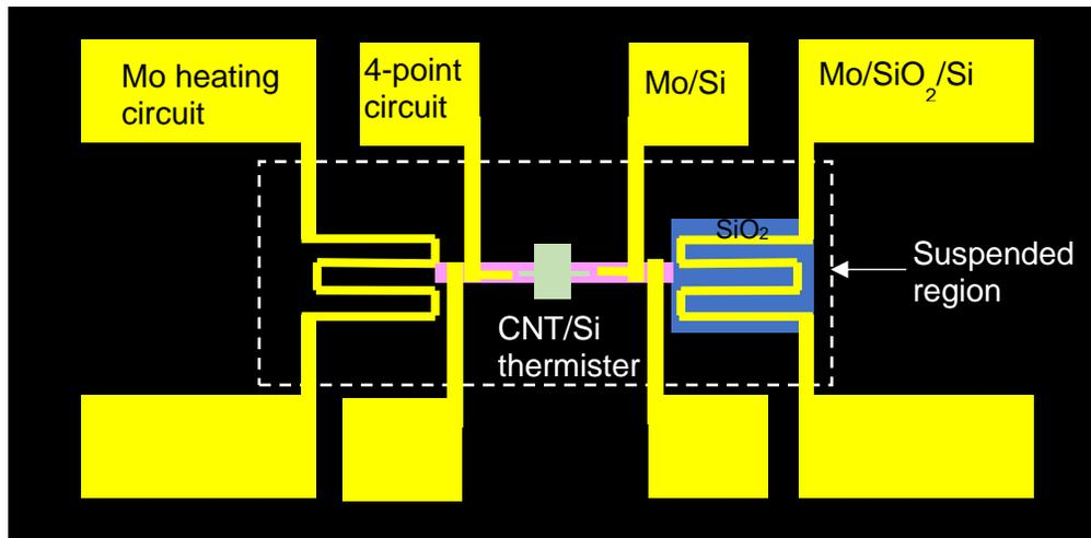
Fig.1 Schematic of the CNT-based microbolometer.
