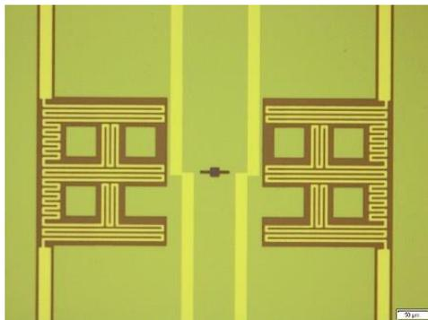
Fig.6 The serpentine Mo heating and sensing circuitry (yellow).
