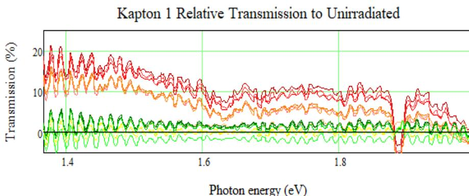
Figure 8: Relative Transmission of Kapton 1 compared to Unirradiated
