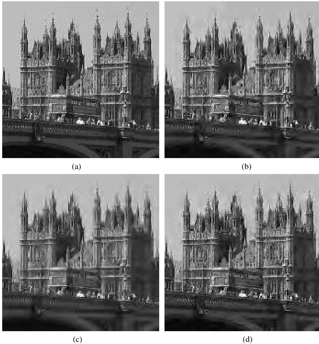
Fig. 2. Portion of the original and encoded London images at bit rate of 0.379 bpp. (a) Original, (b) SPIHT (PSNR = 30.34), (c) SFQ (PSNR = 30.24), and (d) RDVSPIHT (PSNR = 32.03).
