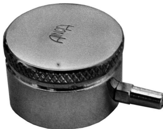
Fig. 1. Metal stethoscope used to house the microphone used for recording the tracheal sounds.
