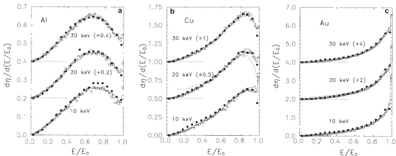
**Figure 5.** Energy distribution of backscattered electrons as a function of  $\epsilon \equiv E/E_0$ . Solid circles are experimental data of Darlington (1975) (normalized so as to give the backscattering coefficient obtained by this author). Dashed lines represent measurements by Matsukawa *et al.* (1974). Histograms are results from the detailed simulation code LEEPS of Fernández-Varea *et al.* (1996). Open circles are results generated with PENELOPE.
