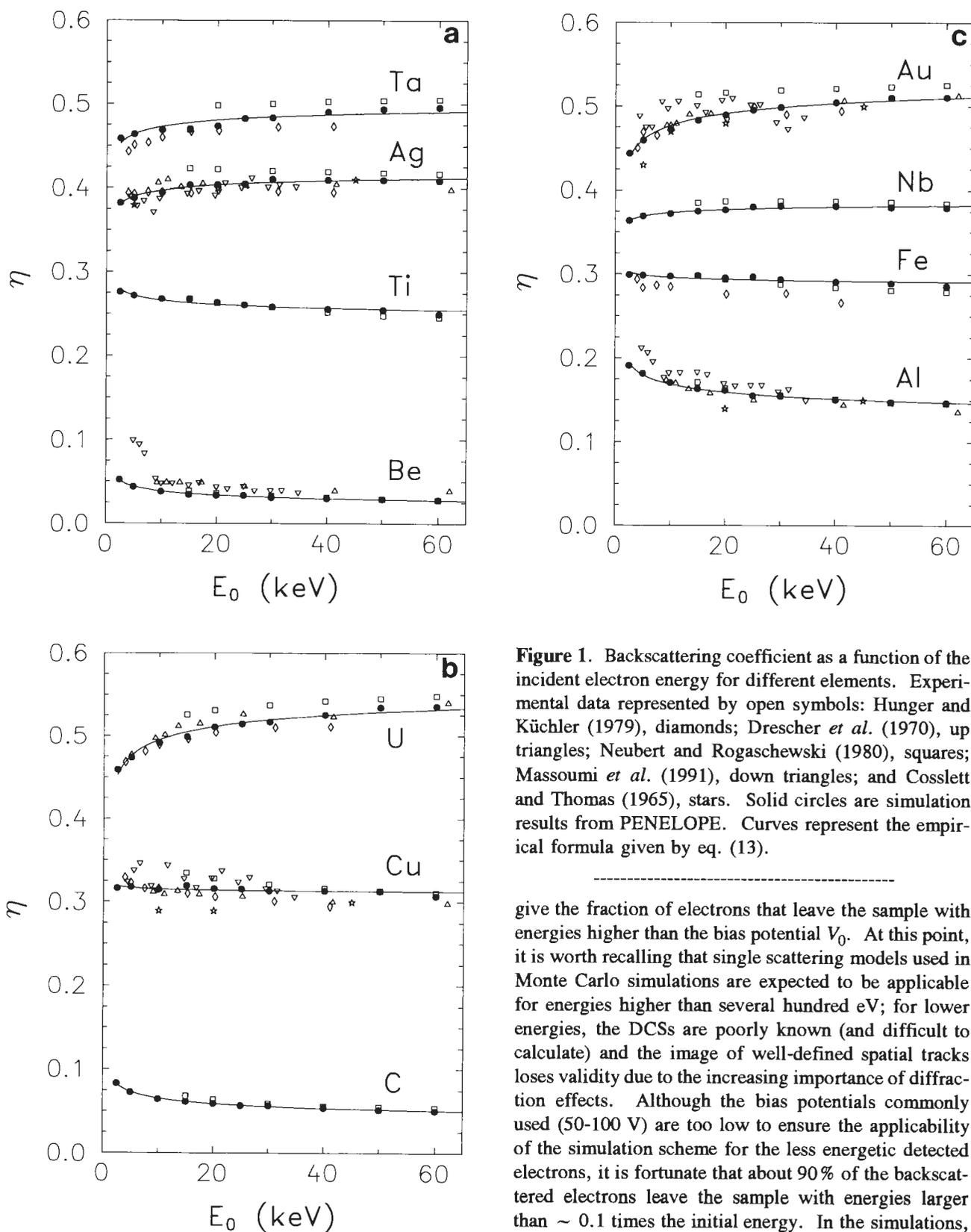
**Figure 1.** Backscattering coefficient as a function of the incident electron energy for different elements. Experimental data represented by open symbols: Hunger and Küchler (1979), diamonds; Drescher *et al.* (1970), up triangles; Neubert and Rogaschewski (1980), squares; Massoumi *et al.* (1991), down triangles; and Cosslett and Thomas (1965), stars. Solid circles are simulation results from PENELOPE. Curves represent the empirical formula given by eq. (13).
