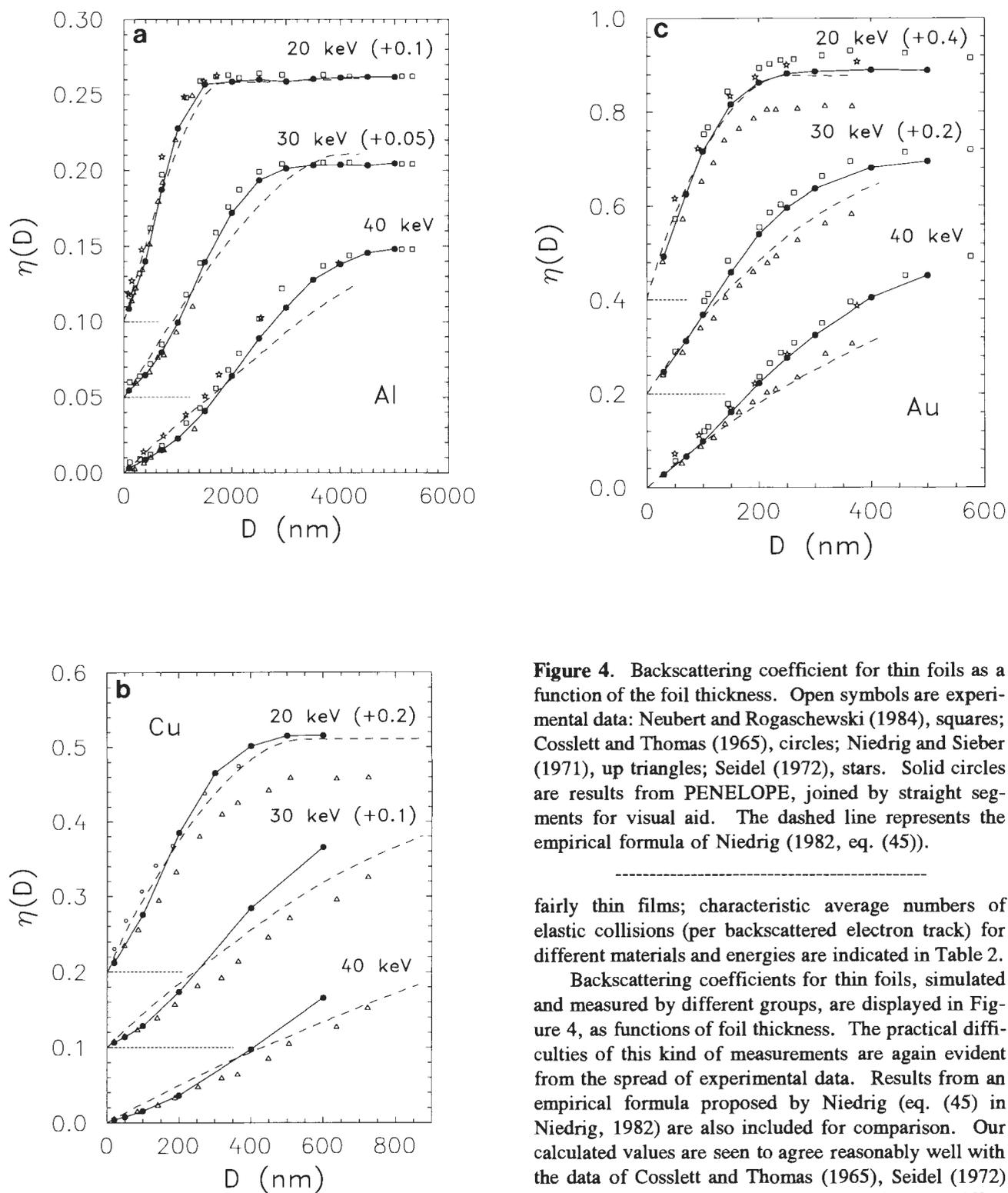
**Figure 4.** Backscattering coefficient for thin foils as a function of the foil thickness. Open symbols are experimental data: Neubert and Rogaschewski (1984), squares; Cosslett and Thomas (1965), circles; Niedrig and Sieber (1971), up triangles; Seidel (1972), stars. Solid circles are results from PENELOPE, joined by straight segments for visual aid. The dashed line represents the empirical formula of Niedrig (1982, eq. (45)).
