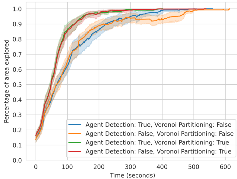
Fig. 4.6: Average area exploration percentage in time for the experiments in LOS scenarios.
