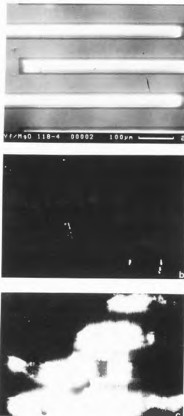
Figure 12. Images of sample A in SE mode (a) and in EBIV mode before (b) and after (c) storage in water for 4000 seconds.
