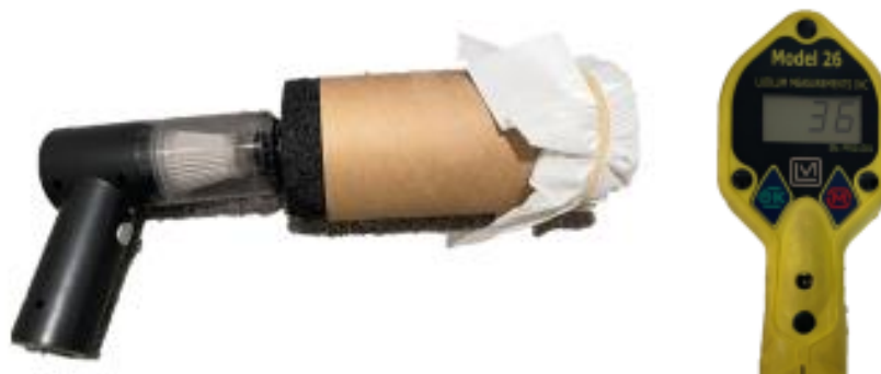
FIG. 2. Some of the equipment that was used for this experiment. On the left, a handheld vacuum with special filter and Kleenex attached with a rubber band. On the right is the Geiger counter used.
