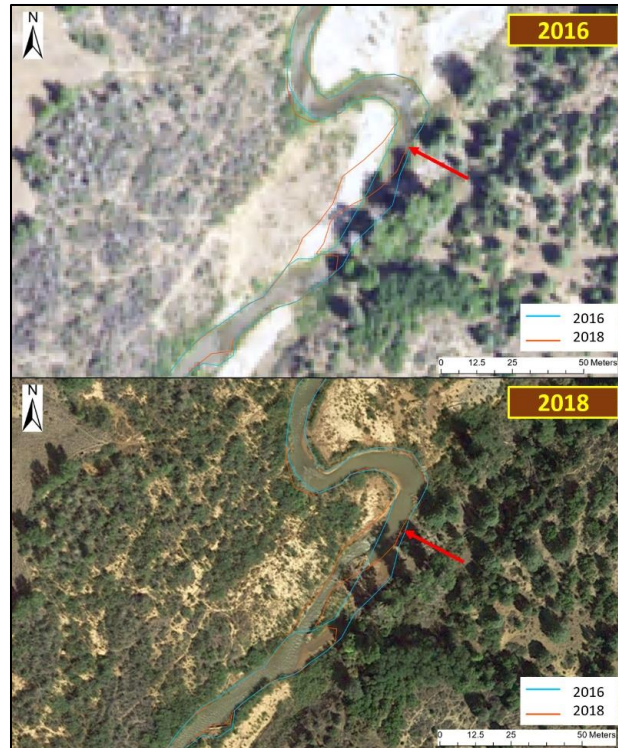
Figure 2.55. Example of bar cutting and bar deposition from 2016-2018 in the Levee reach.
