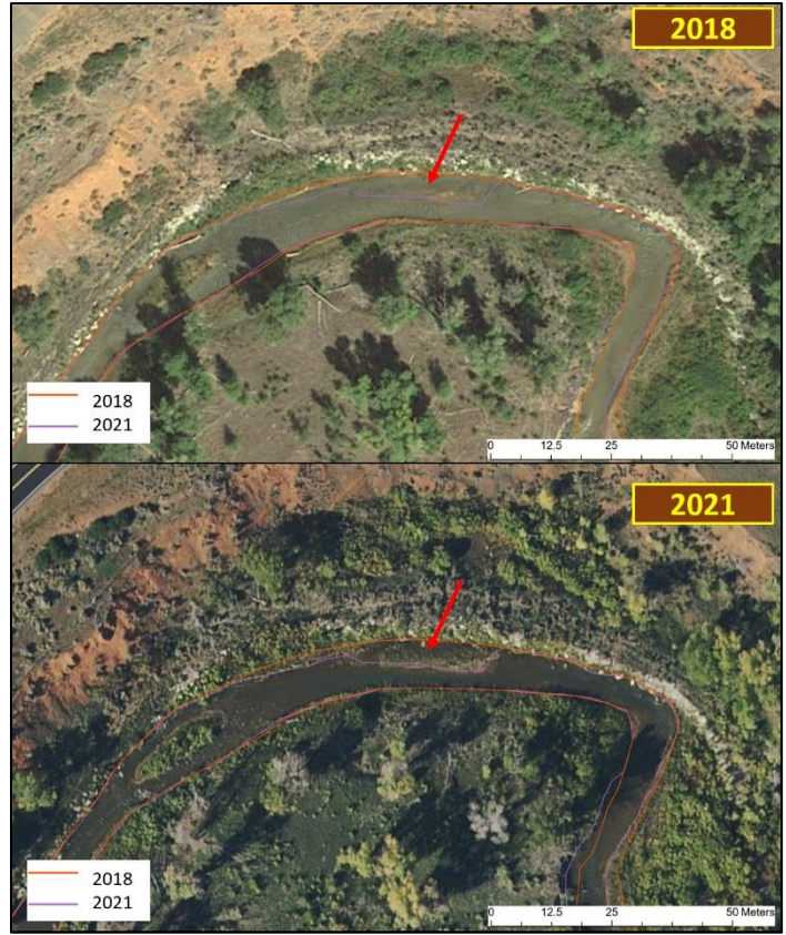
Figure 2.47. Bar deposition between 2018 and 2021 in the lower Oxbow reach.
