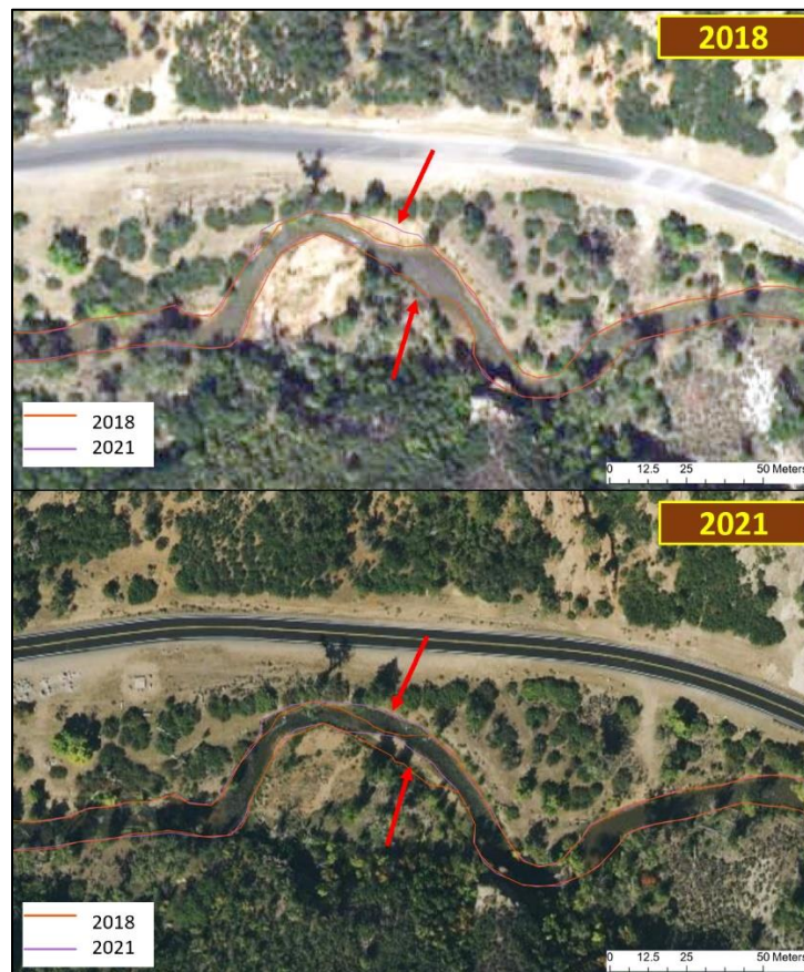
Figure 2.18. Point bar deposition and outer bank erosion in Below Monks Hollow reach at RM 4,800.
