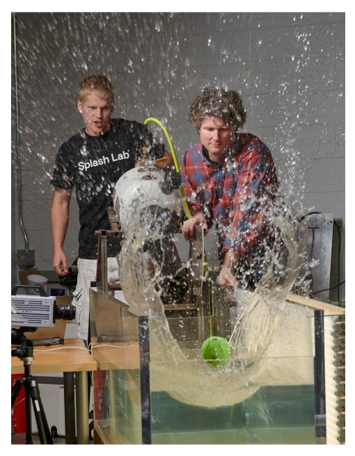
Truscott's study not only reveals the physics of how elastic spheres interact with water, but also predicts how many skips will occur. In addition, the team found that elastic spheres can bounce off the water surface from much higher impact angles compared to rigid spheres – a big clue into why these elastic objects are much easier to skip across the surface.
