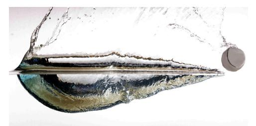
A high-speed camera captured this image of an elastic sphere bouncing off the water surface in a tank. (photo: Chris Mabey)
