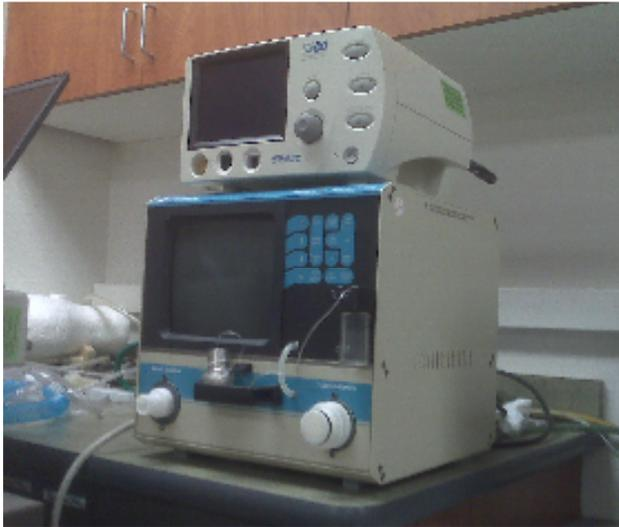
**Figure 3 A size comparison of the NICO<sub>2</sub> (top) and Deltatrac (bottom) metabolic monitors**
