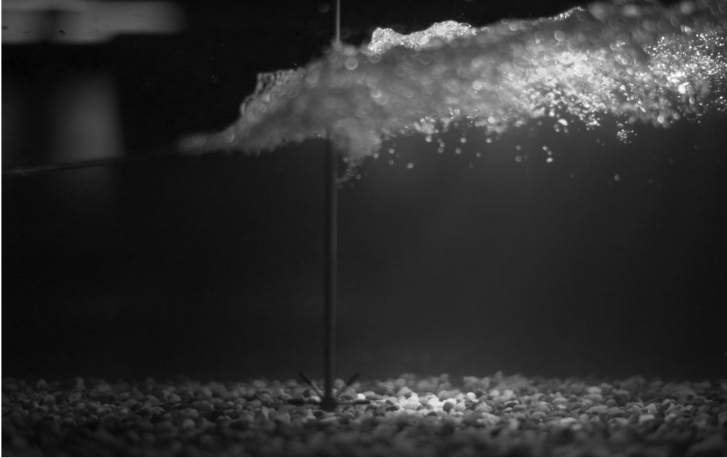
Figure 2. Breaking bore propagating upstream in the experimental channel (exposure time: 7.98 \mu s) - Flow conditions: Q = 0.061 \text{ m}^3/\text{s} , d_1 = 0.1607 \text{ m} , Fr_1 = 1.42
