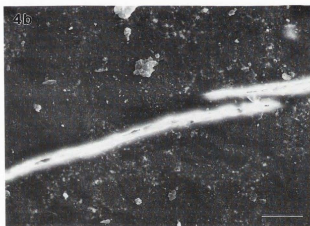
Figure 4. Microcracks growing through bone cement. (a). The BE image clearly differentiates the PMMA beads (circles in cross-section) from the \text{BaSO}_4 containing interbead matrix. Three disconnected "microcracks" are shown. The microcracks appear to have terminated within the PMMA beads (t). The pockmarks on the lower left of the micrograph were caused by beam damage while attempting to photograph at a higher magnification. Bar = 100 \mu\text{m} . (b). The SE image of the microcrack terminations indicated in Figure 4a, at a higher magnification. In this micrograph, it is nearly impossible to differentiate the pre-polymerized beads from the matrix. Bar = 30 \mu\text{m} .
