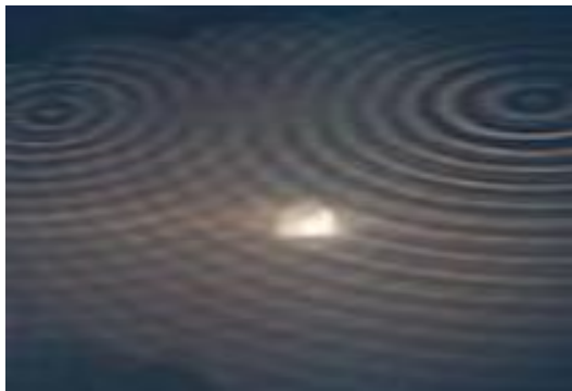
Figure 2: Planar interferences, destructive and constructive, propagating from two quasi point sources showing circular waves centered on the two different point sources. (Source: Wikipedia “interference”)
