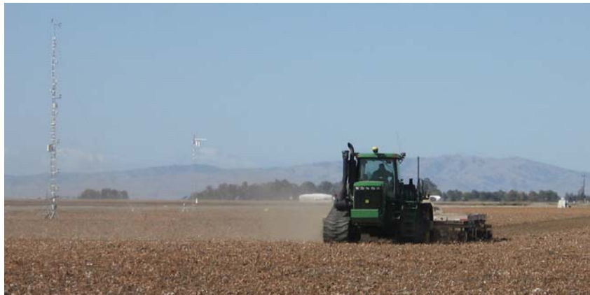
Figure 5. A tractor cultivating a field offers an example of a moving plume. Note the plume and sample towers on the downwind (left) side of the tractor and the Aglite lidar trailer in the distance on the far right.
