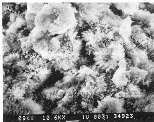
Figures 7-9. Microstructures (formed at 15°C) of: Figure 7. SHAp showing a maximum in interparticulate connectivity for this composition and a high frequency of "donuts." Figure 8. SHAp showing the fine features present within the remnants of the TetCP particles. Figure 9. CDHAp; the interparticulate connectivity appears less than that occurring in samples formed at 37.4°C and the features are not as fine. Bars = 1 \mu m.
