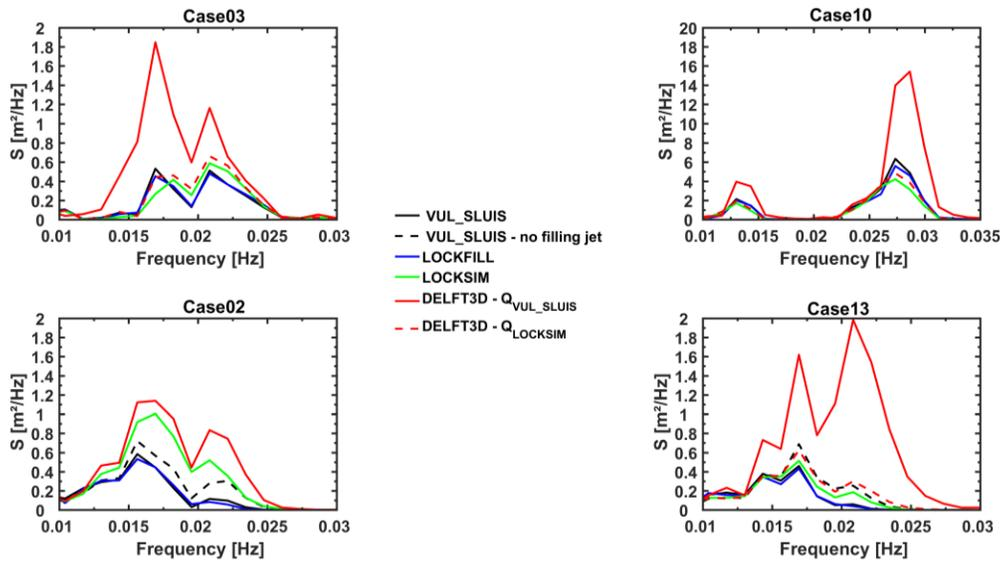
**Figure 7.** Power density spectrum for Case03 (emptying), Case10 (filling only translation waves), Case02 and Case13 (filling multiple force components present).
