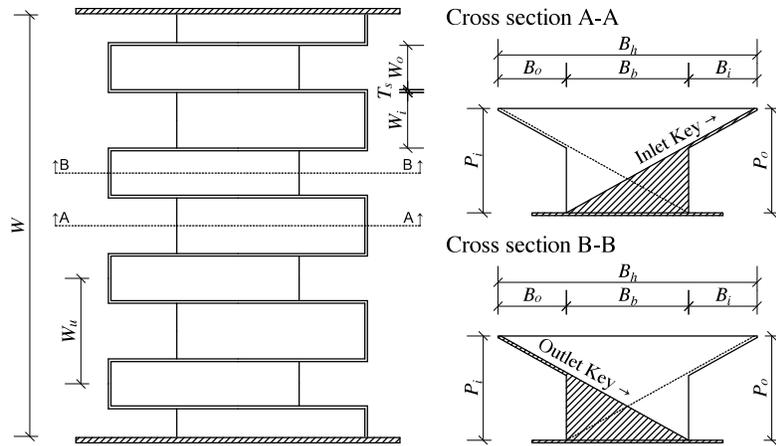
**Figure 1.** Main geometrical PKW parameters, left: plan view, right: sectional view (Oertel and Bremer 2016).
