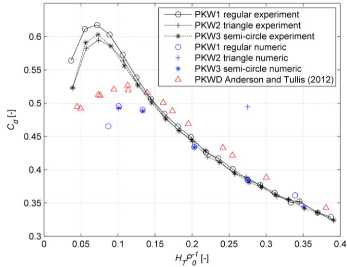
Figure 4. Exemplary discharge coefficients from scaled PKWD model (Oertel 2015).
