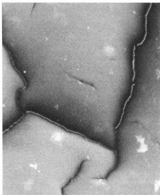
**Figure 1.** Scanning electron micrograph of PLGA 75:25-coated glass coverslip after 14 days in culture medium without cells (37°C, 5% CO<sub>2</sub>) demonstrates cracks on the surface. (White spots are due to salt deposition.) (Field width = 339.6  $\mu$ m).
