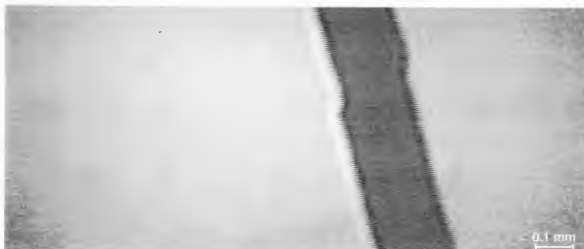
Figure 2. Brewster angle micrograph of C_{16}ISA monolayer on a water surface without applying surface pressure ( \sim 0 mN/m).
