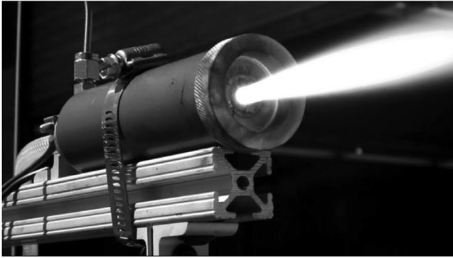
Fig. 13 Flight-weight thruster system during test firing.
