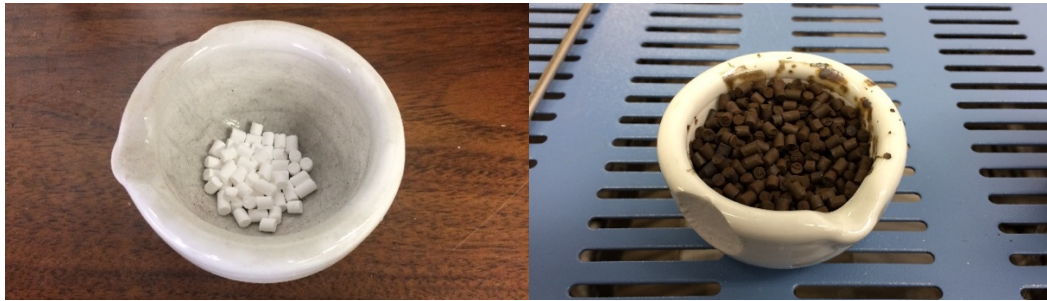
Figure 10: Plain \gamma -Alumina Pellets (Left) and Pellets with \text{MnO}_2 Deposited.
