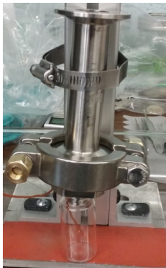
Figure 17: Test Fixture for Measuring Temperature Rise Catalyst Stack.
