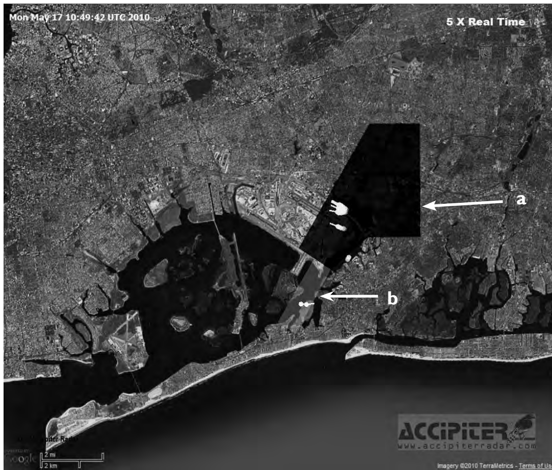
Figure 3. Avian radar alert display for a bird strike discussed in the text for John F. Kennedy International Airport. One safety exclusion zone is marked in black ( a ), indicating “severe” condition, whereas another is gray ( b ), indicating locally “moderate” conditions. The criteria for the safety exclusion zones are set by the airfield biologists and controllers. (Alert zones are colored red and yellow in the actual screen image.)
