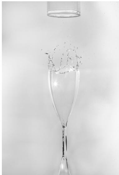
FIG. 1. A high-resolution photograph reveals a thin film of water trailing behind a large mass of water released from a downward-facing tube. The main water mass is below the frame. The film has detached from the tube and collapsed inward (bottom quarter of image). The structure is reminiscent of a champagne flute, with the water column forming the stem and the retracting film forming the bowl. The rim is decorated with satellite droplets from the retreating film border.
