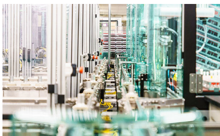
Figure 1: Specimen transport track located in the Automated Core Lab. This picture was taken from online because I was unable to take pictures myself due to HIPPA and HITECH laws. Source: https://www.aruplab.com/news/06-22-15
