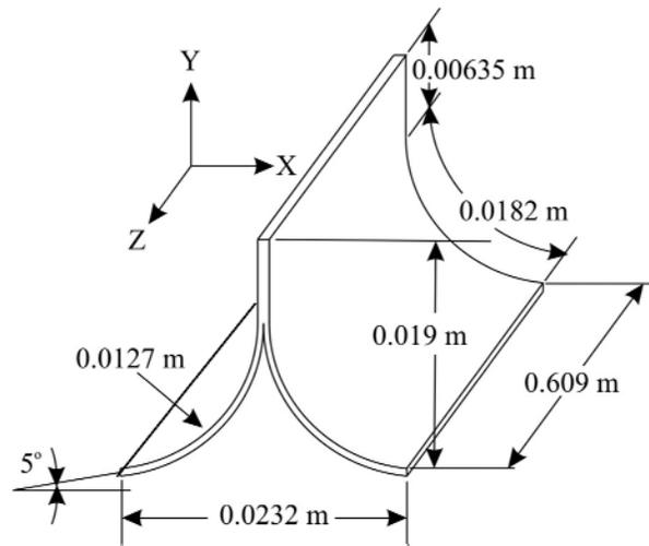
**Figure 6: Dimensions of baseline design, TRACv1.**
