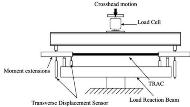
Figure 8: Schematic of four-point bend test device.
