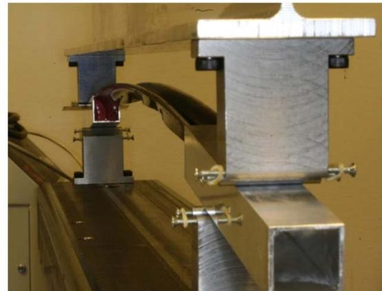
(d) Boom buckled with flanges facing upward
