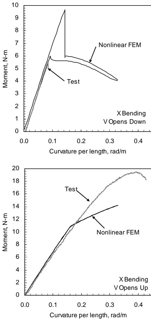
**Figure 11: Nonlinear x axis bending FEM analysis and test results.**
