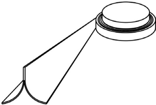
**Figure 4: Deployment of the boom from the stowed position.**
