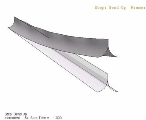
(c) FEM view of boom buckled with flanges facing upward
