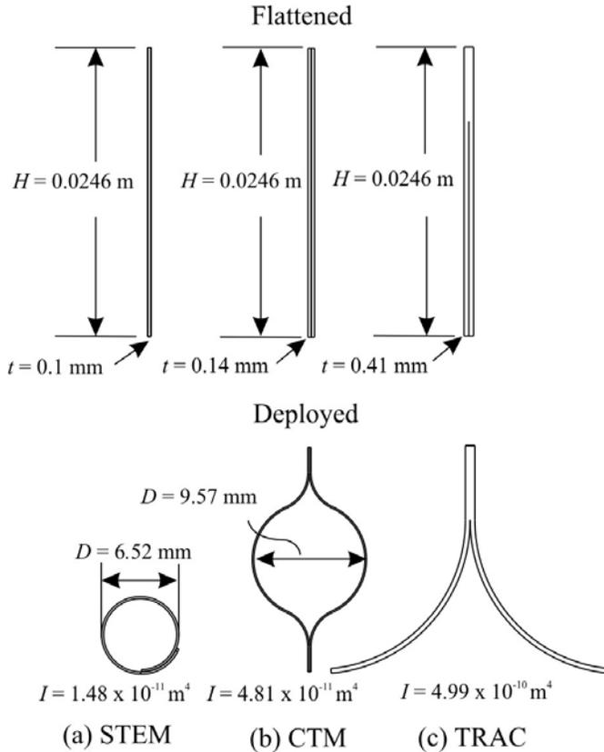
Figure 3: Deployable boom cross-sectional geometry
