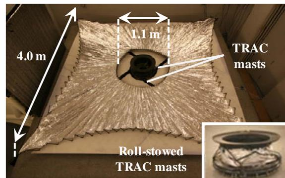
Figure 2: FURL solar sail fully deployed.<sup>2,3</sup>
