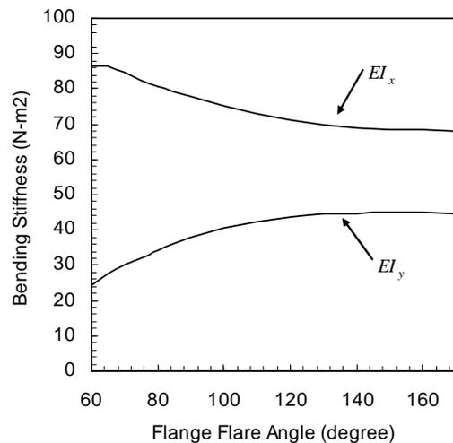
**Figure 7: x and y axis bending stiffness as a function of flare angle for TRACv1.**
