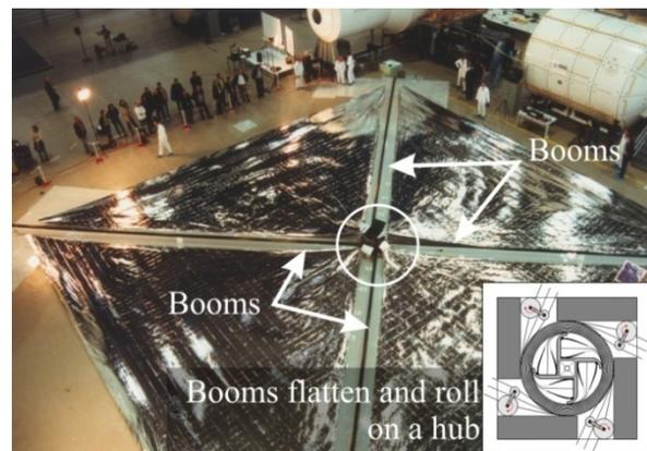
Figure 1: DLR solar sail fully deployed.<sup>1</sup>
