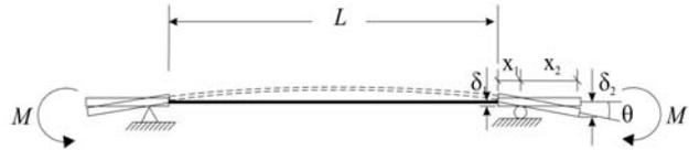
Figure 9: Four-point bend fixture displacements and measurements.
