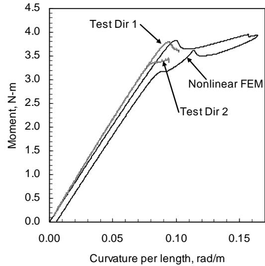
**Figure 12: Nonlinear y axis bending FEM analysis and test results.**
