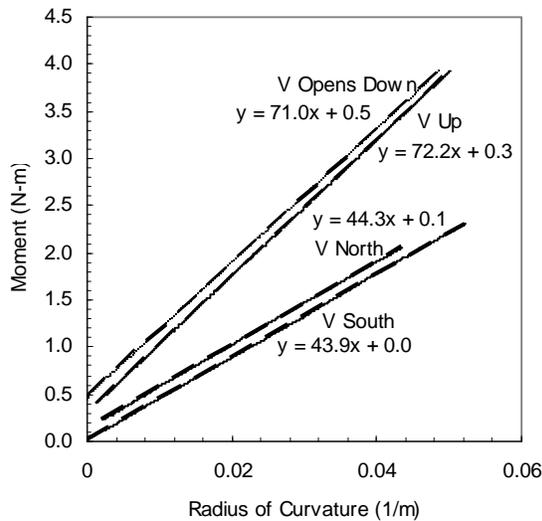
**Figure 15: Moment-curvature response of stiffness bend tests.**
