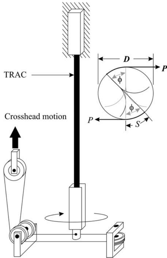
Figure 10: Schematic of the torsion test.
