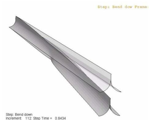
(a) FEM view of boom buckled with flanges facing downward
