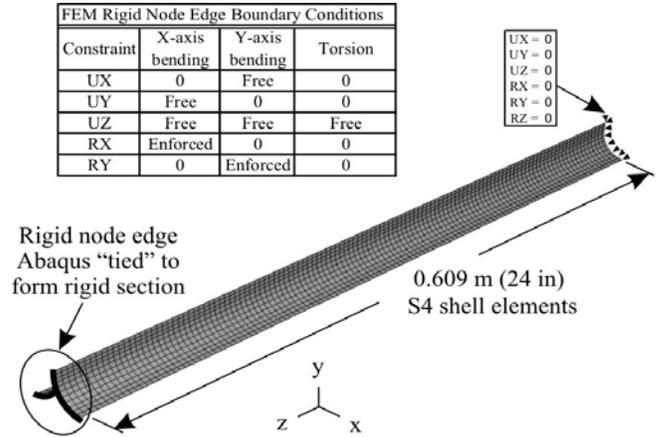
**Figure 5: Boom finite element model boundary conditions.**
