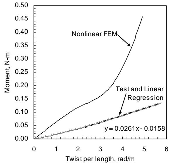
**Figure 13: Nonlinear torsion FEM analysis and test results.**
