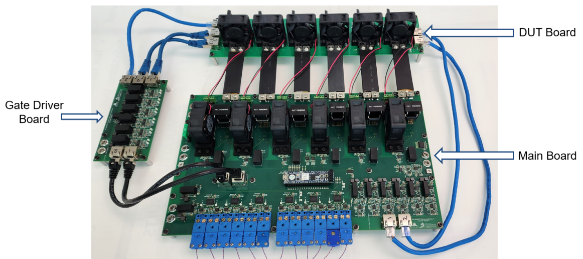
Fig. 4.2: Revision two system with three separate PCBs
