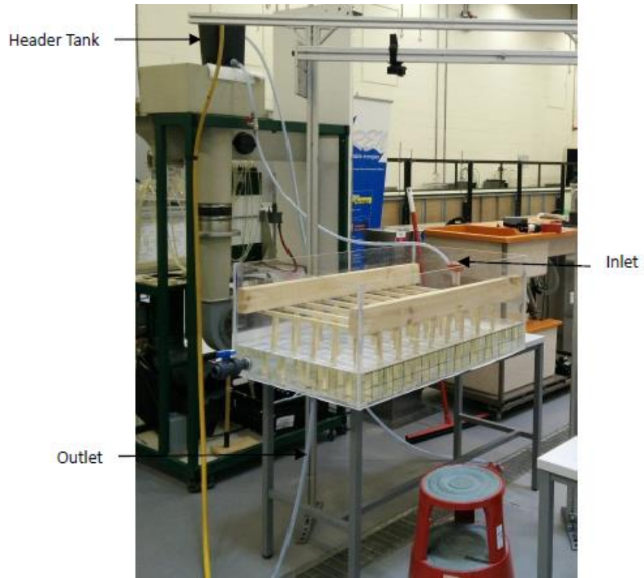
Figure 4. Physical scale model setup in the hydraulics laboratory.
